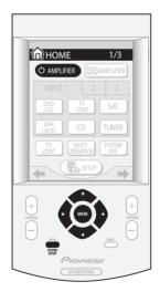
An on-screen display (OSD) appears on your TV. Use the  $\uparrow/\downarrow/(\rightarrow)$  hard keys and **ENTER** on the remote control to navigate through the screens and select menu items.
